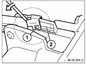
Lift spring (1) off tab (2) on case using a screwdriver and swing upwards.
